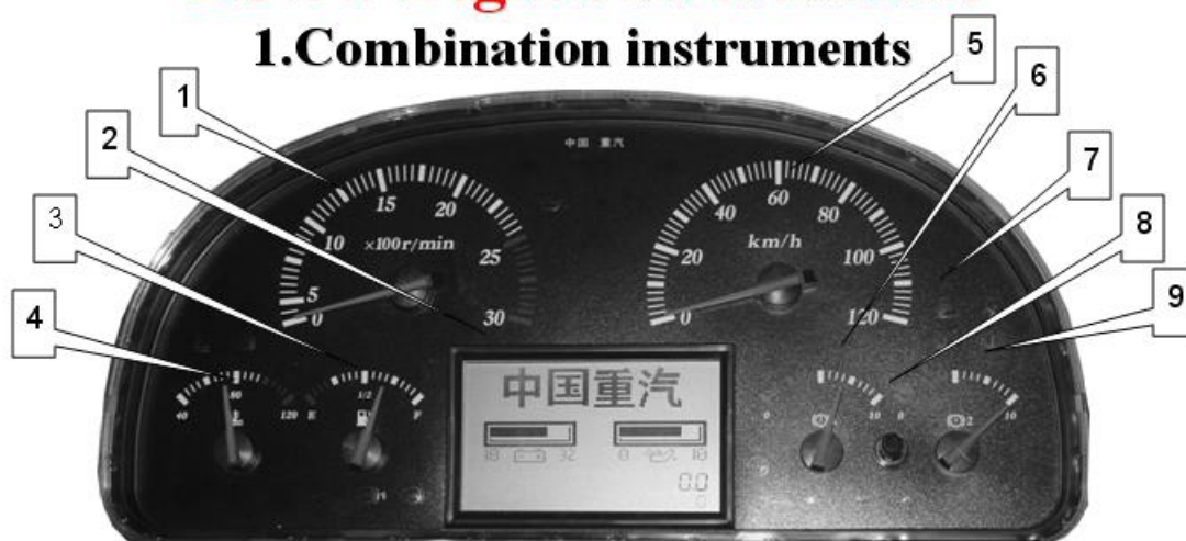
1.Engine tachometer 2.Message display 3.Fuel gauge 4.Water thermometer 5.Speedometer 6.Barometer 1 7.Sign lamp 8.Knob 9.Barometer 2
